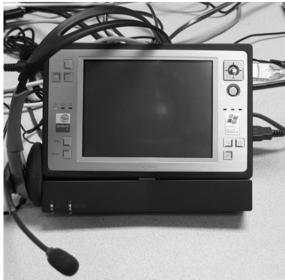
Figure 1. Sony Vaio U71 handheld computer: 4"x3" touch screen.
