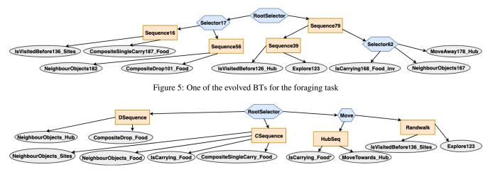
Figure 6: Hand-coded behavior tree for the foraging task
